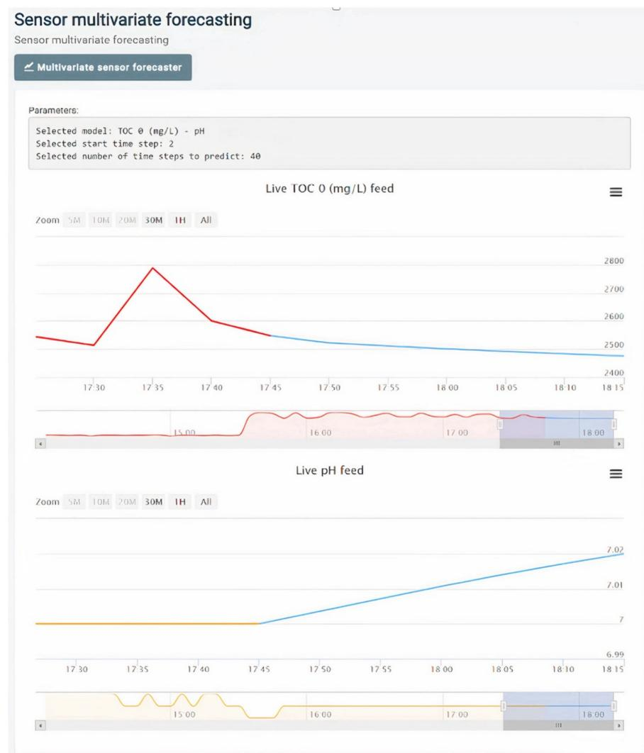
**Figure 5.** Multivariable forecasting, depicted for the TOC measured at the input of the module and the pH of the water. Red (yellow) lines correspond to the values measured for TOC(pH), with blue lines depicting the forecasts of the values.
