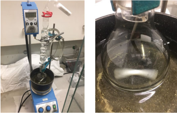
Fig. 10.33 Equipment for solvent debinding
